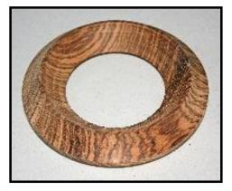
He then reversed the frame onto the 4 jaw chuck and carefully removed the central portion and worked out to the recess. He then
