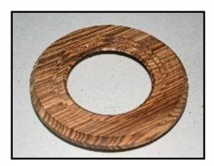
A larger diameter recess was then cut starting on the outside of the original recess, this was to accommodate a backing plate. A small chamfer was turned on the outside edge of the disk. At this point the surface would be sanded through the grits and an oil finish applied (but as this was a demo Tom skipped this).
